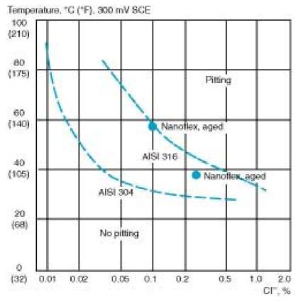
Figure 1: Critical pitting temperatures (CPT) for Nanoflex $^{\text{\tiny M}}$ , ASTM 304 and ASTM 316 at varying concentrations of sodium chloride. Potentiostatic determinations at +300 mV (SCE), pH = 6.0.
