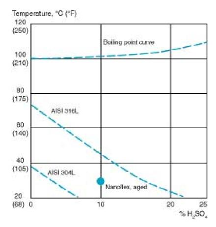
Figure 2: Isocorrosion diagram for Nanoflex<sup>™</sup>, ASTM 304L and 316L in stagnant sulfuric acid. The curves for ASTM 304L and 316L and the dot for Nanoflex<sup>™</sup> represent a corrosion rate of 0.1 mm/year.
