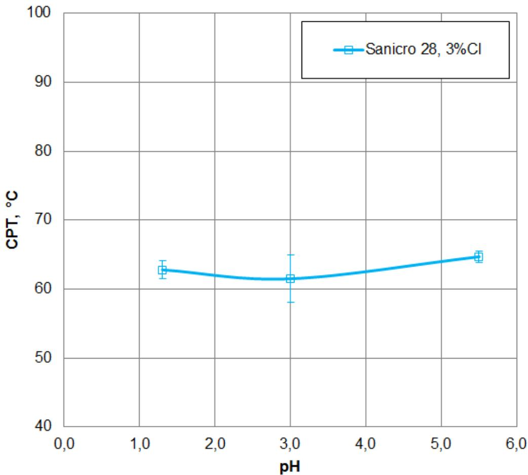
Figure 2. Critical pitting temperature (CPT) as a function of pH for cold worked Sanicro® 28 in a 3% Cl<sup>-</sup> solution. The potential was +634 mV vs Ag/AgCl.
