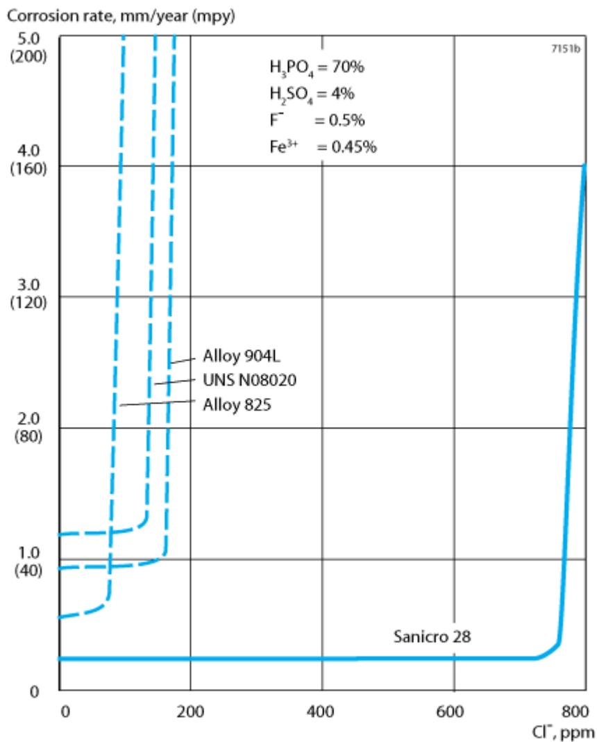
Figure 1. Corrosion rate in contaminated phosphoric acid at different chloride concentrations 100°C (210°F). Comparison of Sanicro® 28 and other alloys (chemical compositions given in table 1).
