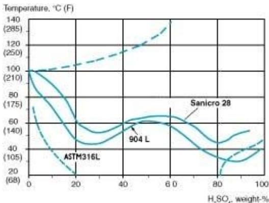
Figure 3. Isocorrosion diagram for Sanicro® 28, Alloy 904L and ASTM 316L, in deaerated sulfuric acid. The curves
