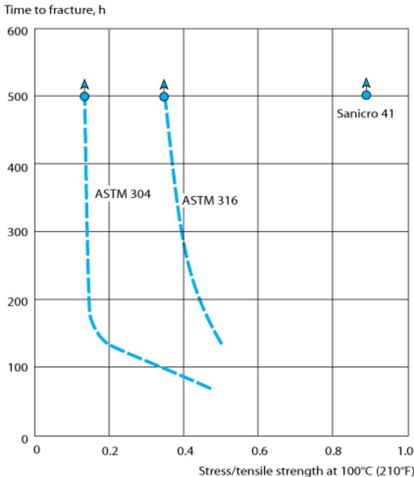
Figure 3. Results of stress corrosion cracking tests in 40 % CaCl<sub>2</sub> at 100 °C (210 °F), pH=6.5.
