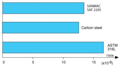
Figure 2. Thermal expansion per °C (30-100°C).
