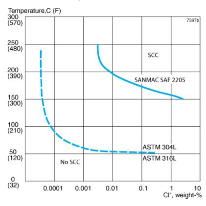
Figure 3. Resistance to stress corrosion cracking (SCC) in neutral chloride solutions with an oxygen content of 8 ppm. Laboratory results for Sanmac 2205 of constant load specimens loaded to the proof strength at the test temperature.
