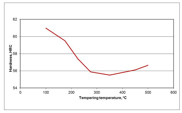
Brittleness and loss of corrosion resistance occur with tempering above 450°C (840°F).
