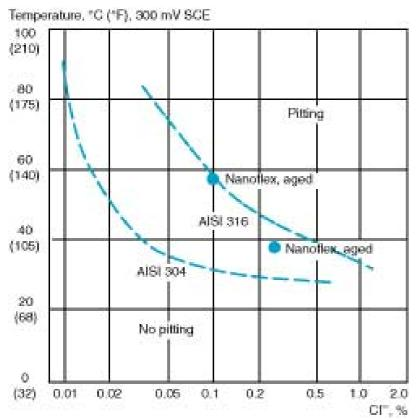
Figure 1: Critical pitting temperatures (CPT) for Nanoflex<sup> $^{\times}$ </sup>, ASTM 304 and ASTM 316 at varying concentrations of sodium chloride. Potentiostatic determinations at +300 mV (SCE), pH = 6.0.
