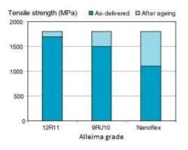
Figure 3. As delivered tensile strength needed to reach the same final tensile strength of about 1850 MPa after ageing in Nanoflex<sup>™</sup> compared to two other spring steel grades.
