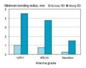
Figure 4. Minimum bending radius at as delivered tensile strength according to figure 3. Testing has been made across and along the rolling direction (RD). Strip thickness 0.5 mm.
