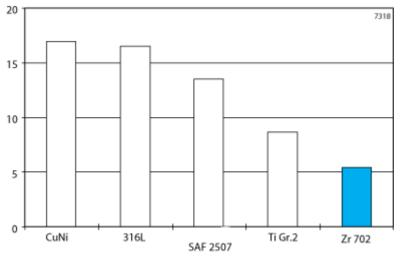
Figure 3 Thermal expansion vs. material.
