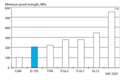
Figure 1 Yield strength vs. tubing material.
