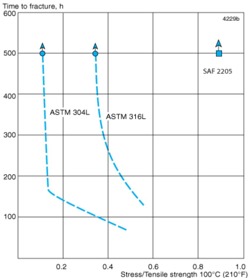
Figure 8. Results of stress corrosion cracking (SCC) tests on SAF™ 2205, ASTM TP304L and ASTM TP316L in 40% CaCl<sub>2</sub>, pH 6.5, at 100°C (210°F) with aerated test solution.
