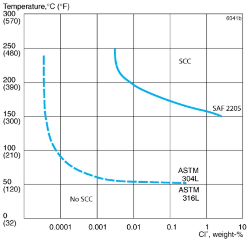
Figure Figure 7. Resistance to stress corrosion cracking (SCC) in neutral chloride solutions with an oxygen content of about 8 ppm. Laboratory results for SAF™ 2205 of constant load specimens loaded to the proof strength at the test temperature.
