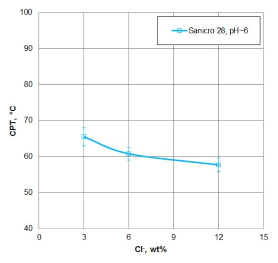
Figure 1. Critical pitting temperature (CPT) as a function of chloride concentrations for cold-worked Sanicro<sup>®</sup> 28. The potential was +634 mV vs Ag/AgCl.
