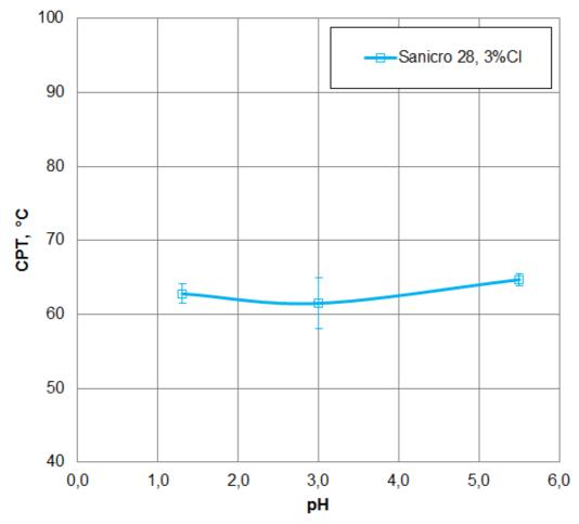
Figure 2. Critical pitting temperature (CPT) as a function of pH for cold worked Sanicro<sup>®</sup> 28 in a 3% CI- solution. The potential was +634 mV vs Ag/AgCI.
