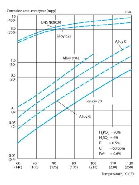
Figure 2. Corrosion rate in contaminated phosphoric acid at different temperatures for Sanicro® 28 and some other alloys (chemical compositions given in table 1).
