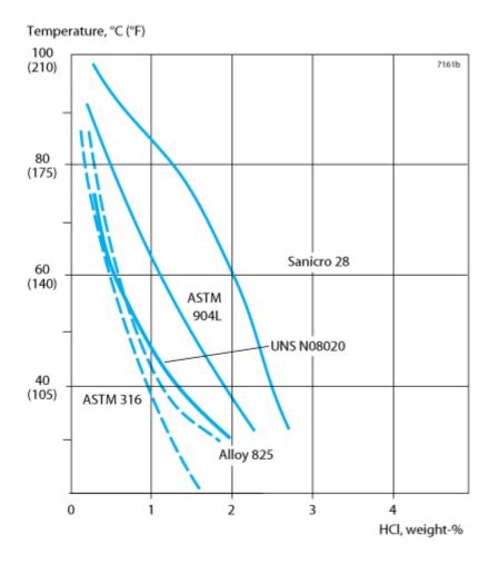
Figure 5. Isocorrosion in hydrochloric acid. The curves repesent a corrosion rate of 0.1 mm/year (4 mpy).
