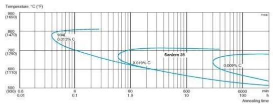
Figure 11. TTC diagram for Sanicro® 28 with two different carbon contents and for Alloy 904L (Alleima 2RK65). The curves repesent normal limit values for the carbon content.
