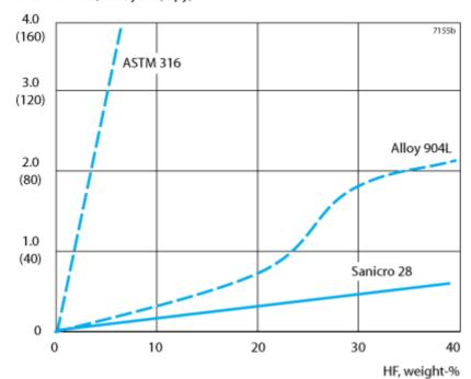
Figure 6. Corrosion rates in hydrofluoric acid at 20°C (68°F) for Sanicro® 28, Alloy 904L and AISI 316.
