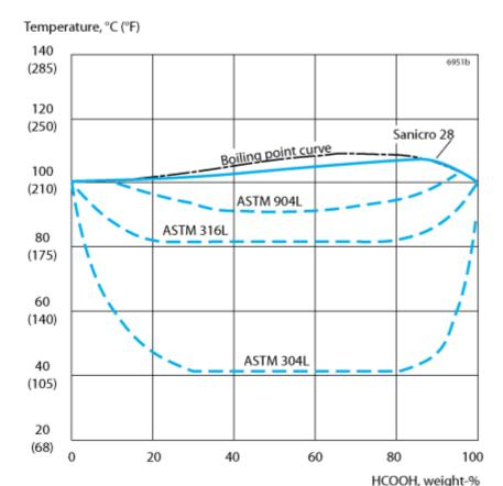
Figure 7. Isocorrosion diagram for Sanicro® 28 and other alloys in formic acid at a corrosion rate of 0.1 mm/year (4 mpy).
