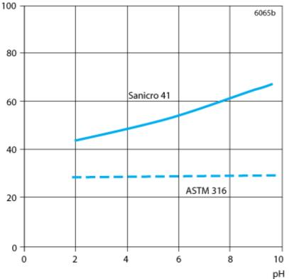
Figure 2. Critical pitting temperatures for Sanicro 41 and AISI 316 in 3 % NaCl solutions at different pH values.
