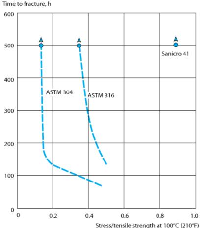
Figure 3. Results of stress corrosion cracking tests in 40 % CaCl<sub>2</sub> at 100 °C (210 °F), pH=6.5.
