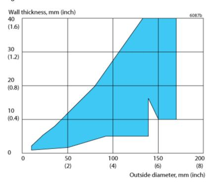
Figure 1. Principal size range for seamless tube and pipe.
