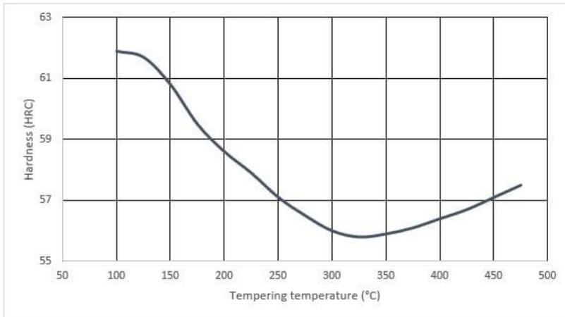
Below is an estimation of the hardness levels that can be expected with different tempering temperatures.
