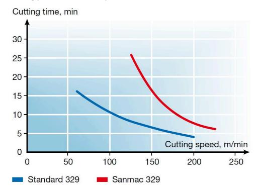
By applying the collective Sanmac knowledge in the upgrade of the standard Alloy 329, Alleima R&D engineers have increased the machinability of the material to a new level. That, combined with a low spread in the manufacturing process, will provide major benefits to customers using Sanmac 329.
