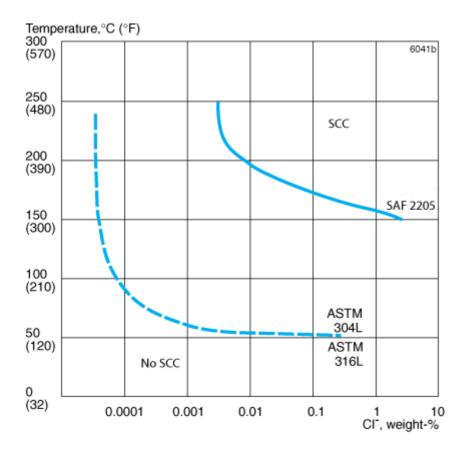
Figure Figure 7. Resistance to stress corrosion cracking (SCC) in neutral chloride solutions with an oxygen content of about 8 ppm. Laboratory results for SAF<sup>™</sup> 2205 of constant load specimens loaded to the proof strength at the test temperature.
