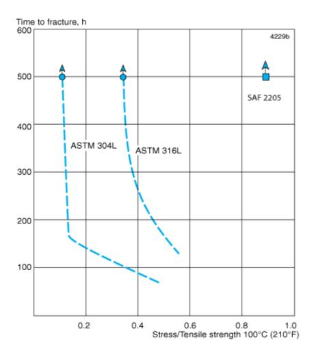
Figure 8. Results of stress corrosion cracking (SCC) tests on SAF<sup>™</sup> 2205, ASTM TP304L and ASTM TP316L in 40% CaCl<sub>2</sub>, pH 6.5, at 100°C (210°F) with aerated test solution.
