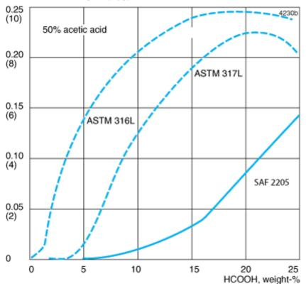
Figure 4. Corrosion rate of SAF<sup>™</sup> 2205, ASTM TP316L and ASTM TP317L in boiling mixtures of 50% acetic acid and varying proportions of formic acid. Test time 1+3+3 days.
