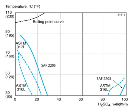
Figure 3. Iso- corrosion diagram for SAF<sup>™</sup> 2205, ASTM TP316L and ASTM TP317L in sulphuric acid. The curves represent a corrosion rate of 0.1 mm/year (4 mpy) in a natural aerated stagnant test solution.
