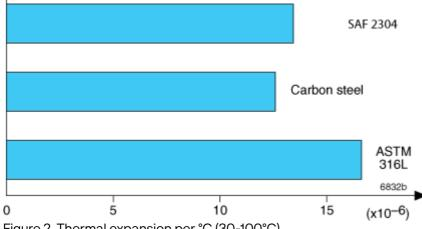
Figure 2. Thermal expansion per °C (30-100°C).
