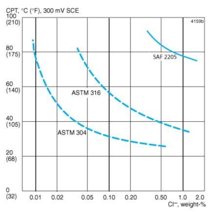
Figure 6. Critical pitting temperatures (CPT) for SAF<sup>™</sup> 2205, ASTM TP304 and ASTM TP316 at varying concentrations of sodium chloride (potentiostatic determination at +300 mV SCE), pH6.0
