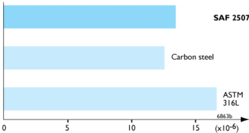
Figure 3. Thermal expansion, per °C (30-100°C, 86-210°F).
